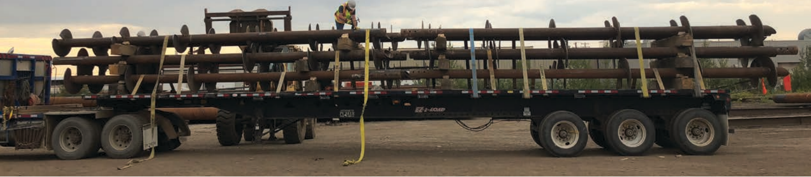
A loaded truck of screw piles
